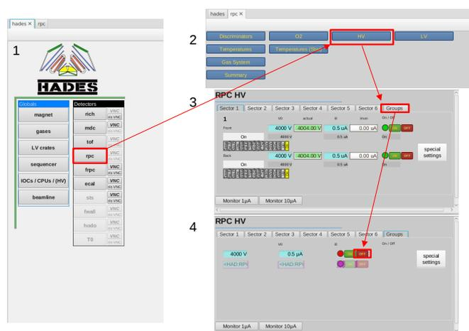
Figure 10: RPC HV off procedure
