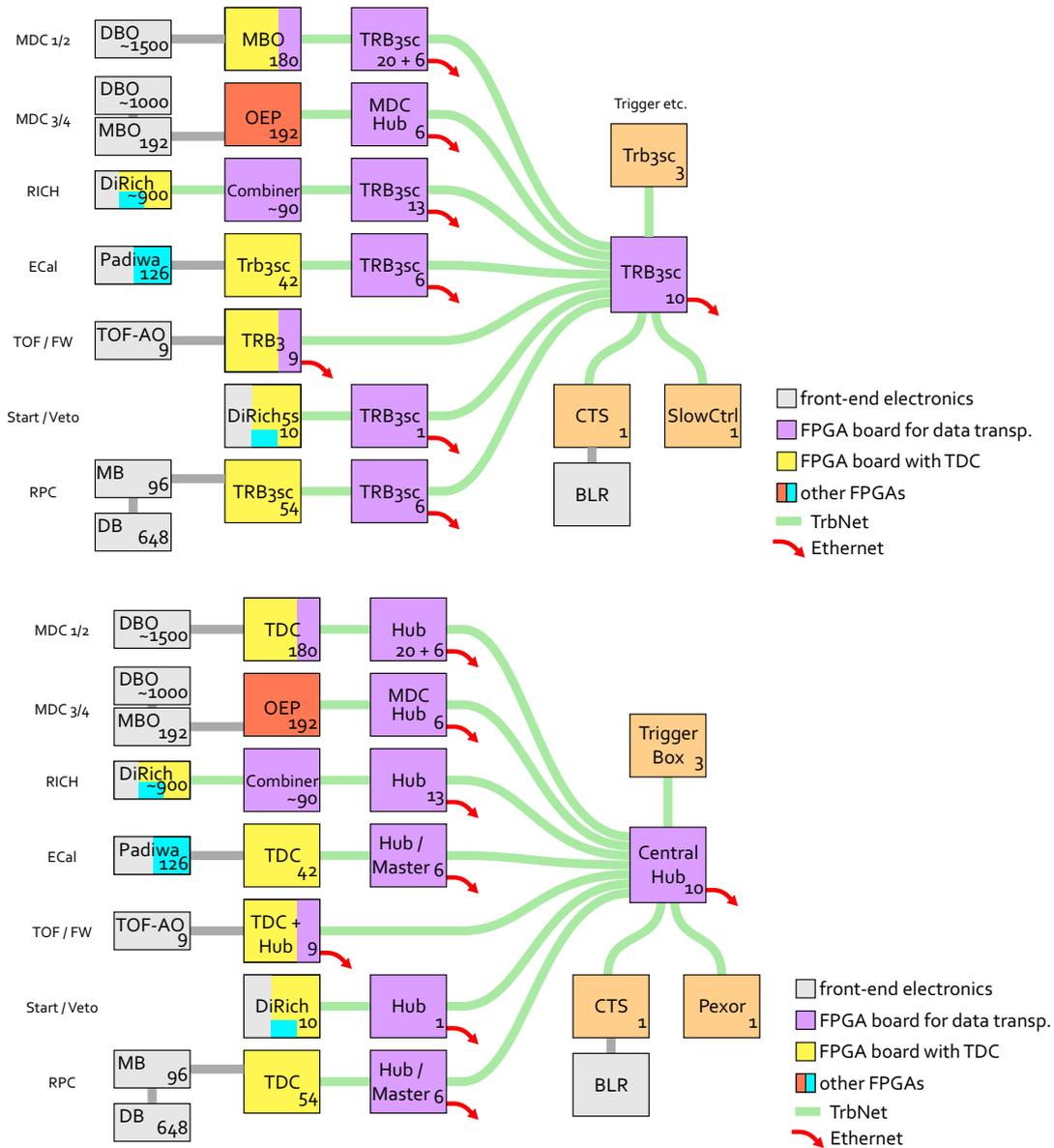
Figure 4: DAQ network with different labels. Labels by type of board and by function (names as often shown in Hmon). Numbers show the amount of boards in Hades
