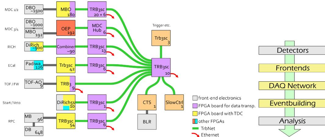
Structure of DAQ - red arrows point towards the eventbuilder computers. Right: simplified data flow view
